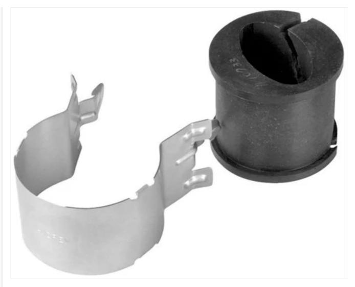
This image displays the two primary components of the Commscope EWSH-52 Waveguide Snap-in Hanger Kit: a silver-colored metal clamp designed to secure the waveguide, and a black, cylindrical rubber insert that provides cushioning and a snug fit for the waveguide within the clamp.
