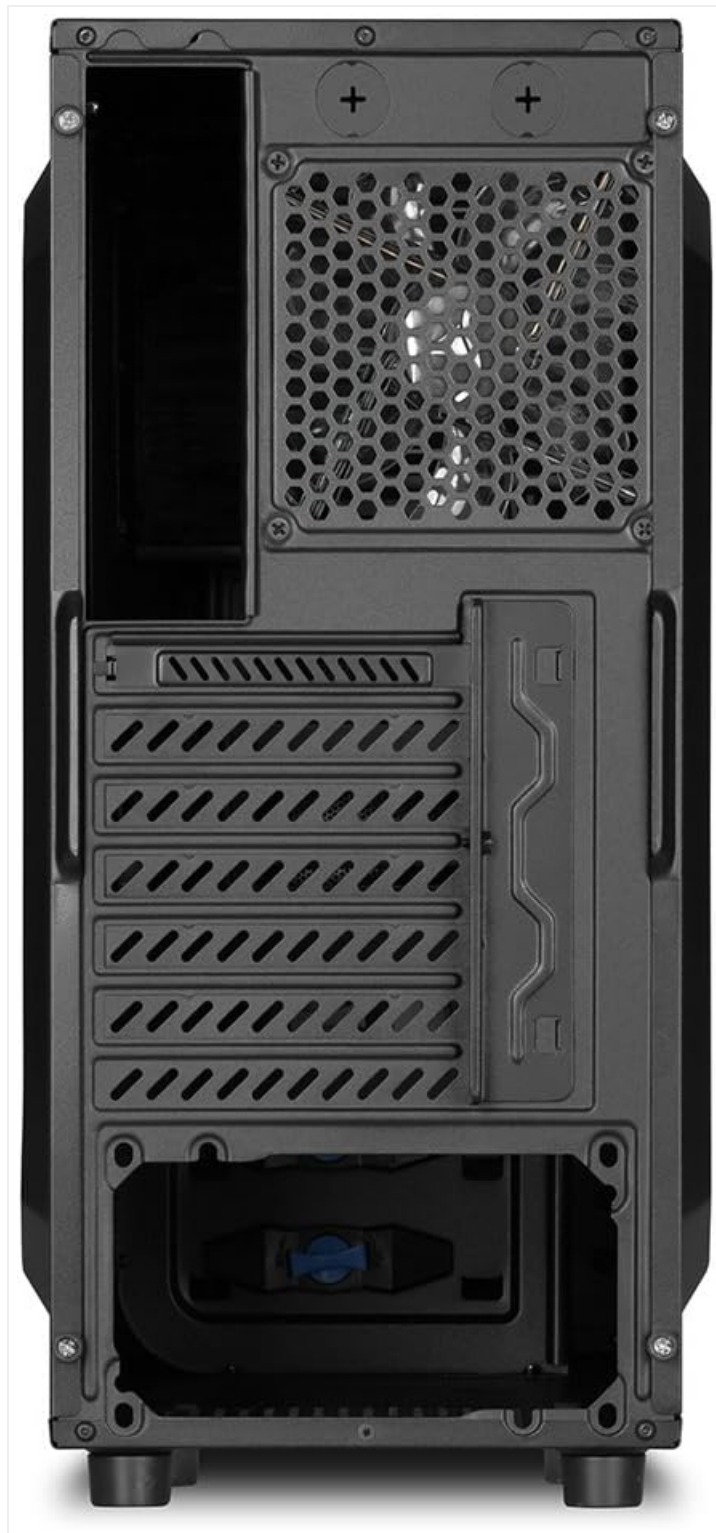
Figure 2.3: Rear Panel. This view shows the back of the case, including the cutout for the motherboard I/O shield, seven PCI expansion slots, and the pre-installed 120mm rear fan.
