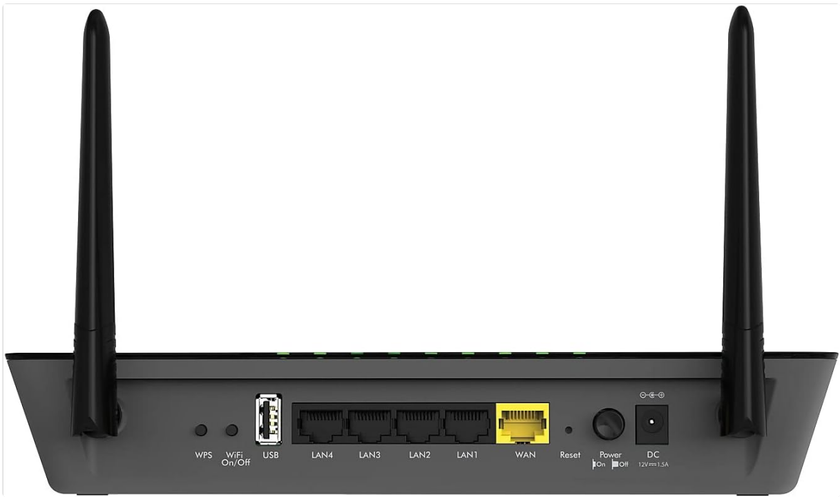
Image: Rear view of the NETGEAR R6220 AC1200 Smart Wi-Fi Router, showing the various ports and buttons including WPS, USB, LAN, WAN, Reset, Power On/Off, and DC power input.
