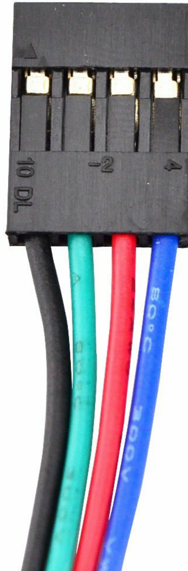
Figure 4.2: 4-pin connector for the stepper motor.
