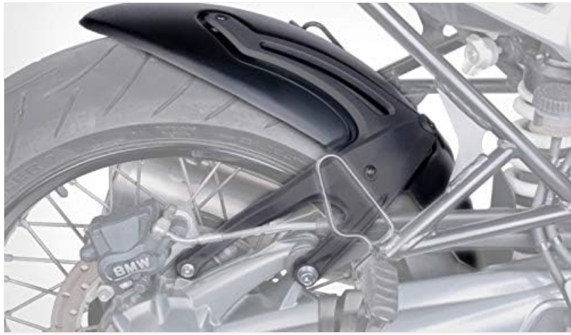
Figure 2: The Puig 7023J Rear Fender shown installed on a BMW R Nine T series motorcycle, illustrating its position relative to the rear wheel and suspension.
