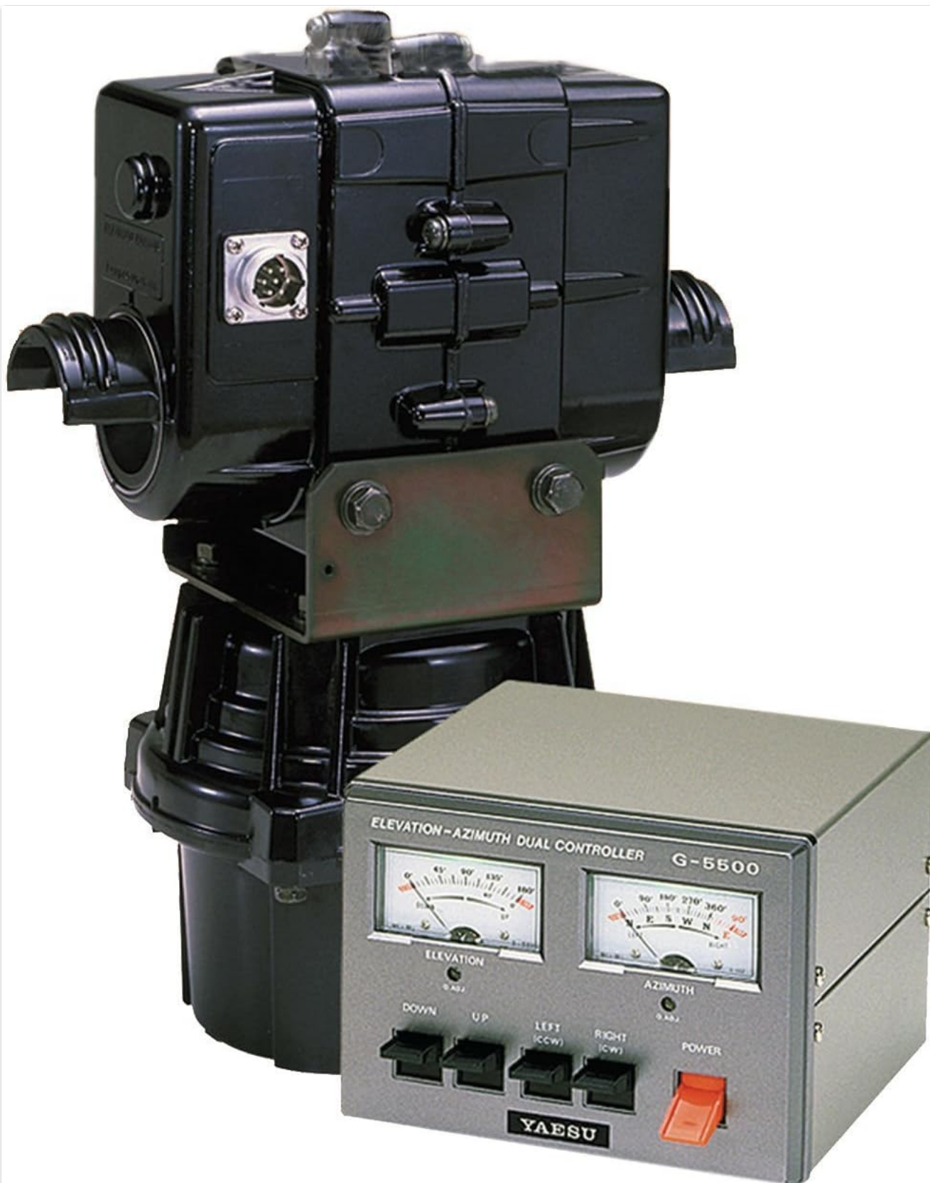
Figure 1: Yaesu G-5500 Azimuth-Elevation Rotator unit (left) and Control Box (right). The rotator unit connects to the control box via two 6-conductor cables (not shown). The control box features dual meters for elevation and azimuth, along with directional control switches and a power switch.
