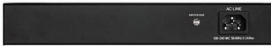
Figure 4: Rear panel of the DGS-1016C showing the power input and grounding screw.
