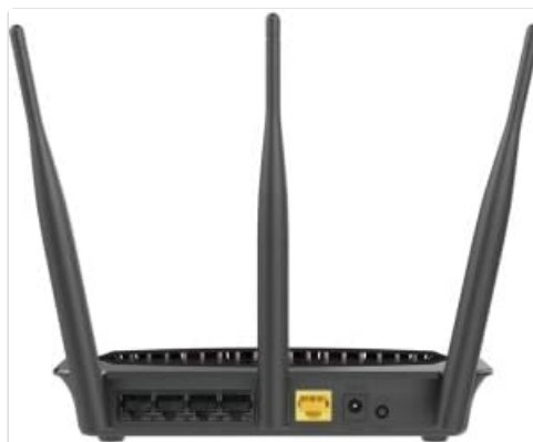
Figure 2: Rear view of the D-Link DIR-813 router. This image displays the back of the router, showing the power input, WAN port (yellow), four LAN ports, and a WPS/Reset button.
