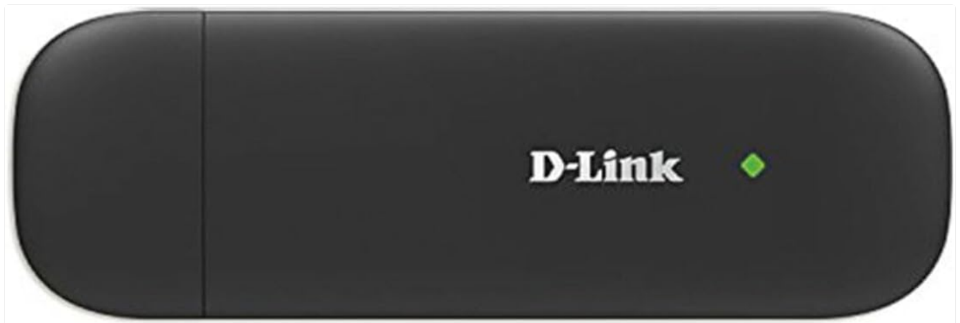
Figure 1.1: Front view of the D-Link DWM-222 4G LTE USB Adapter, showing the D-Link logo and an LED indicator.
