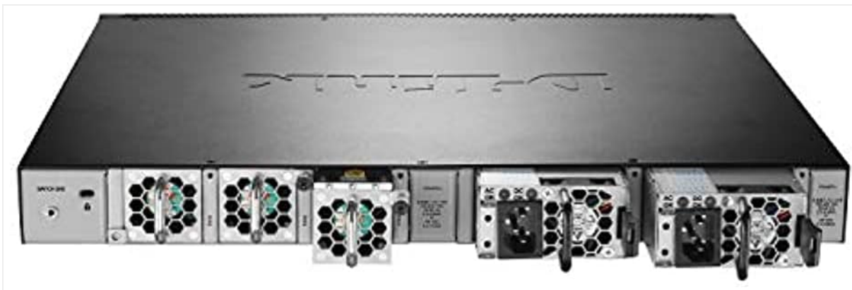
Figure 4.3: Rear panel view of the D-Link DXS-3400-24SC switch. This view highlights the modular power supply bays, typically supporting redundant power supplies for enhanced reliability. Multiple cooling fan modules are also visible, designed for efficient heat dissipation. The grounding screw is located on the left side.
