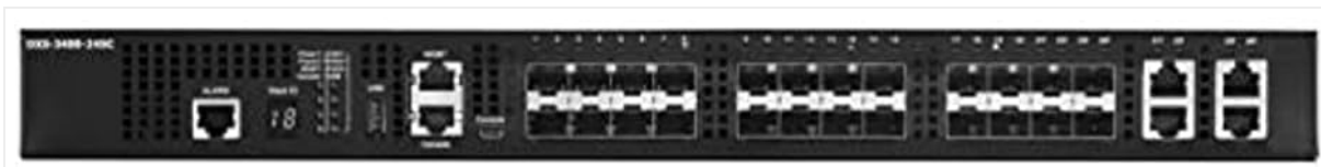
Figure 4.2: Detailed front panel view of the D-Link DXS-3400-24SC switch. From left to right, the front panel includes system status LEDs (Power, Alarm, Link/Act), a console port (RJ-45), a USB port, and then the twenty (20) SFP+ ports followed by four (4) combo RJ45/SFP+ ports. Each port has its own link/activity LED.
