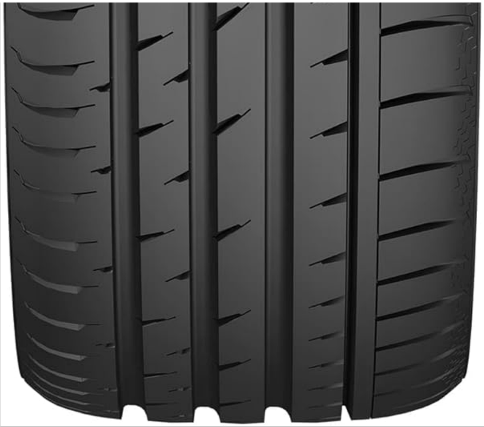
Figure 4: Close-up of tire tread, highlighting the grooves for water dispersion and grip.
