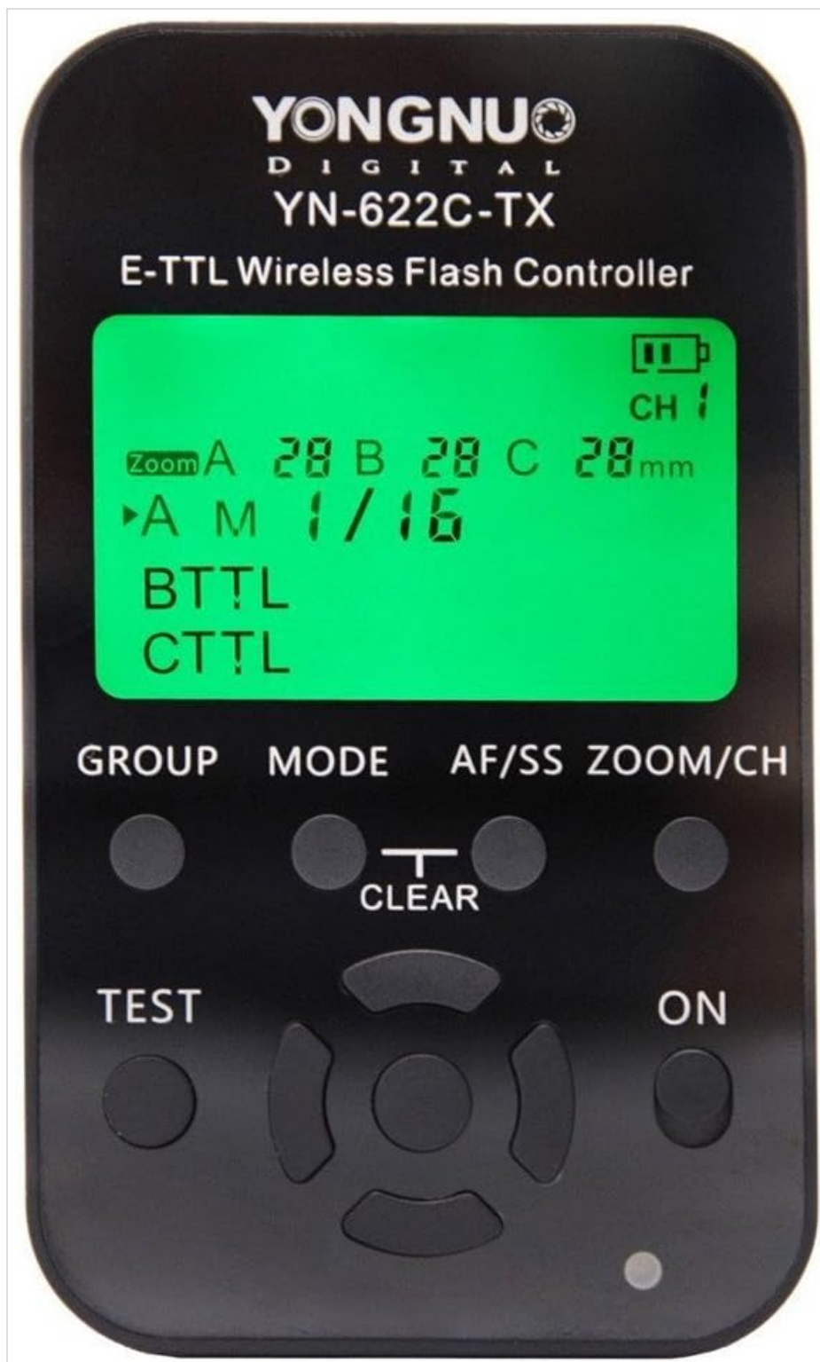
Figure 2.1: Front view of the YN622C-TX controller, displaying its LCD screen and control buttons. The screen shows group settings (A, B, C), flash modes (E-TTL, Manual, Super Sync), and channel information.
