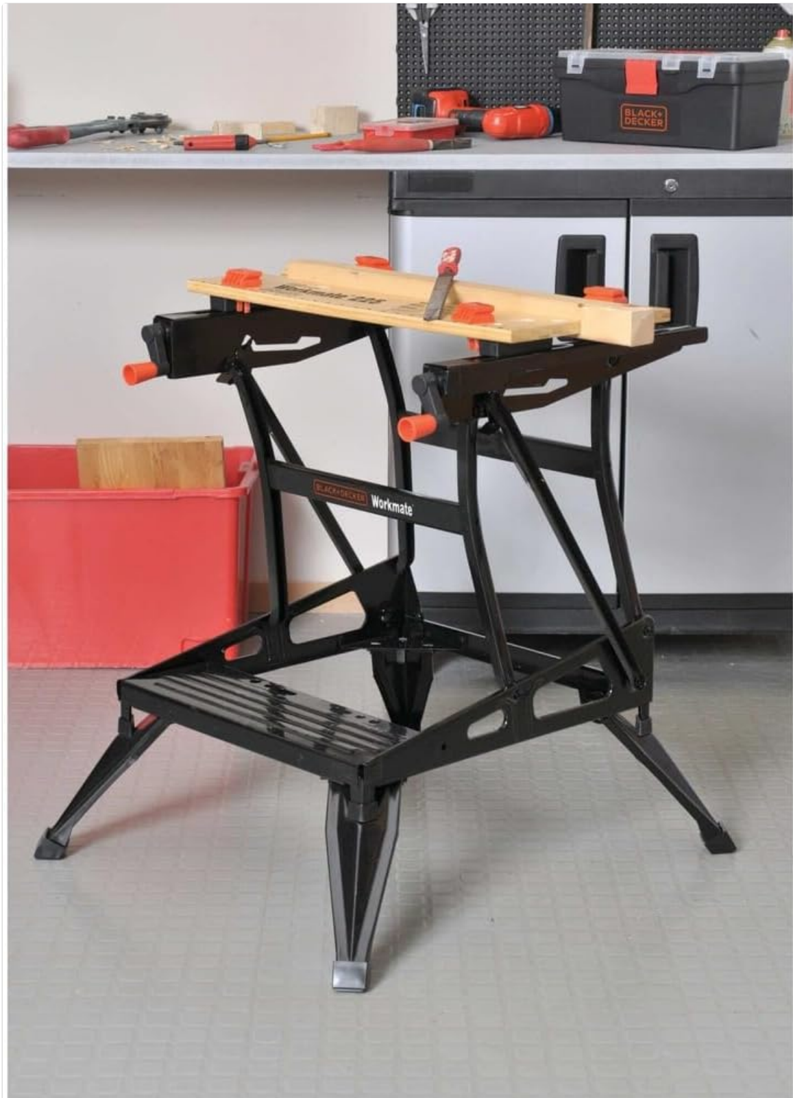
Figure 5.1: A piece of wood being clamped between the adjustable jaws.
