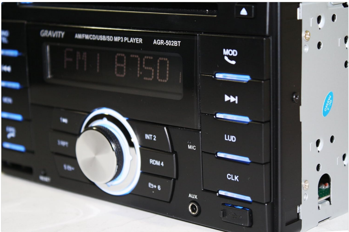
Image: Detailed view of the Gravity AGR-502BT front panel, highlighting the display, control knob, and various function buttons such as CLK, MOD, and BND/TEL.
