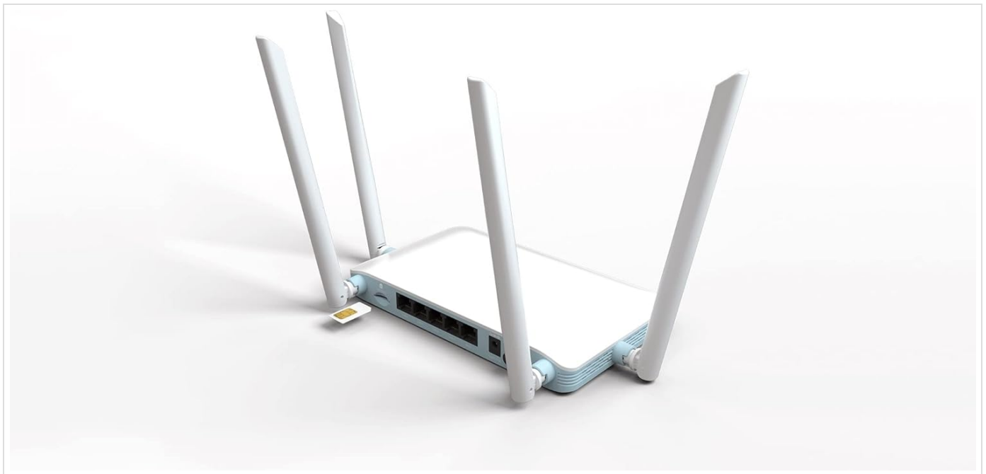
Figure 3.3: Detailed view of the SIM card slot on the D-Link G403/E router, showing how a SIM card is inserted.
