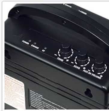
Figure 3: Top panel controls for audio adjustment.
