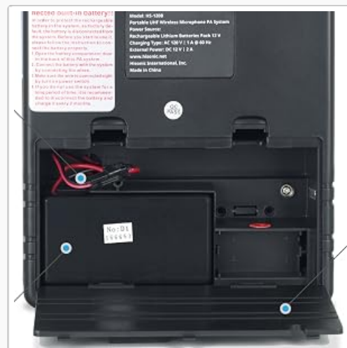
Figure 4: Rear panel with battery compartment access.
