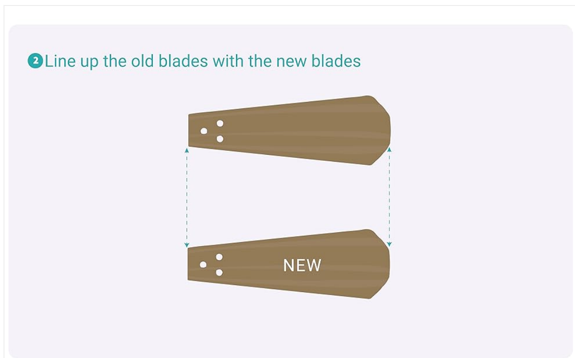
Image 4: Lining up old and new fan blades. This image depicts an old fan blade placed directly over a new blade, demonstrating how to compare their shapes and hole patterns.
