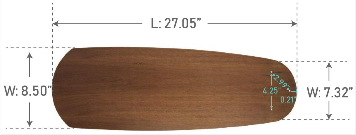
Image 2: Craftmade B570E-WB6 Fan Blade Dimensions. This image illustrates the precise measurements of the fan blade, including its length (L: 27.05"), maximum width (W: 8.50"), minimum width (W: 7.32"), and the spacing of the pre-drilled holes (4.25", 2.99", 0.22").
