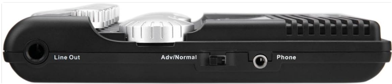
Figure 5: Side view showing the Line Out, Adv/Normal switch, and Phone output.
