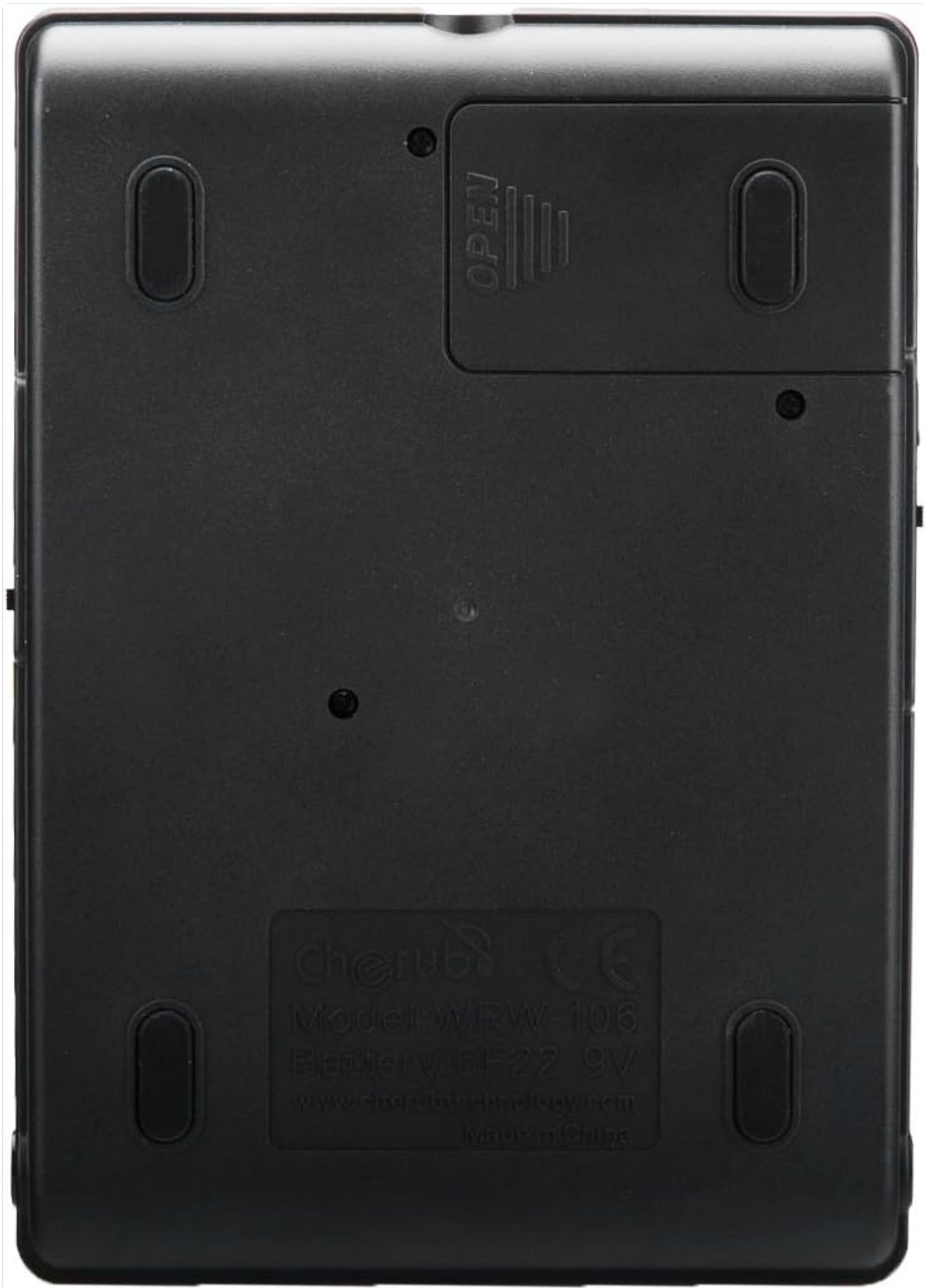
Figure 2: Back view of the WRW-106, highlighting the battery compartment.
