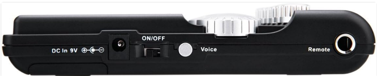
Figure 4: Side view showing the DC IN 9V port, ON/OFF switch, Voice button, and Remote input.
