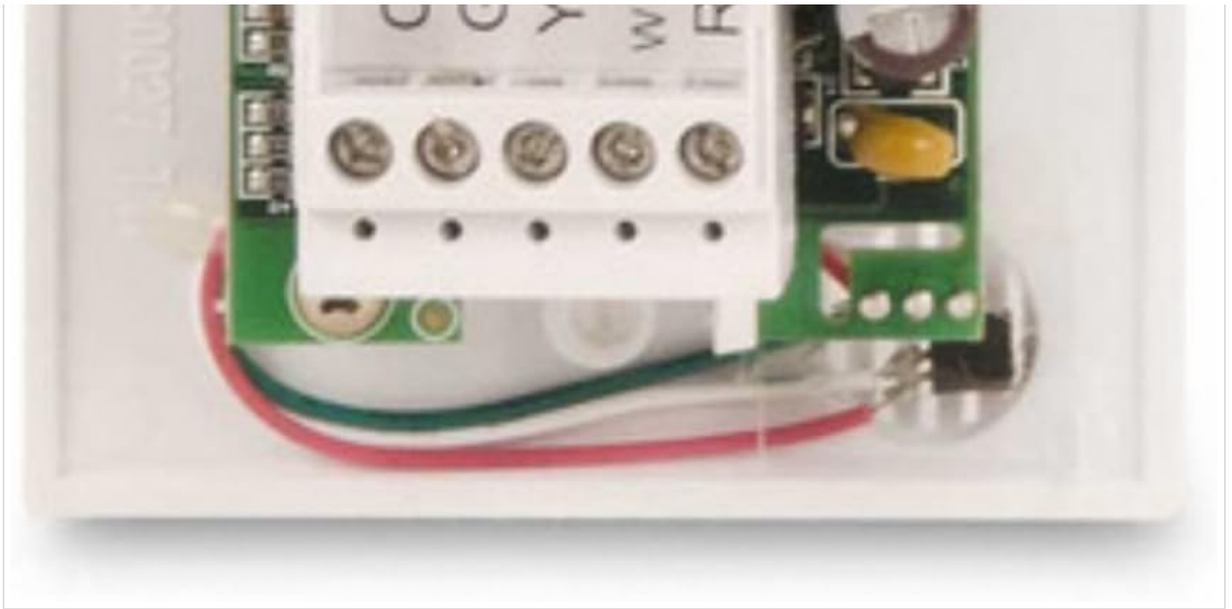
Figure 2: Rear view of the thermostat, illustrating the wiring terminal block for HVAC system connections.
