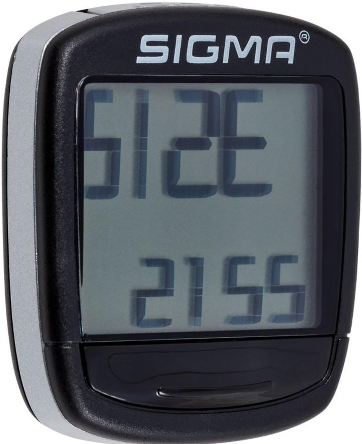
Figure 3.3: The display indicating the wheel size setting mode.
