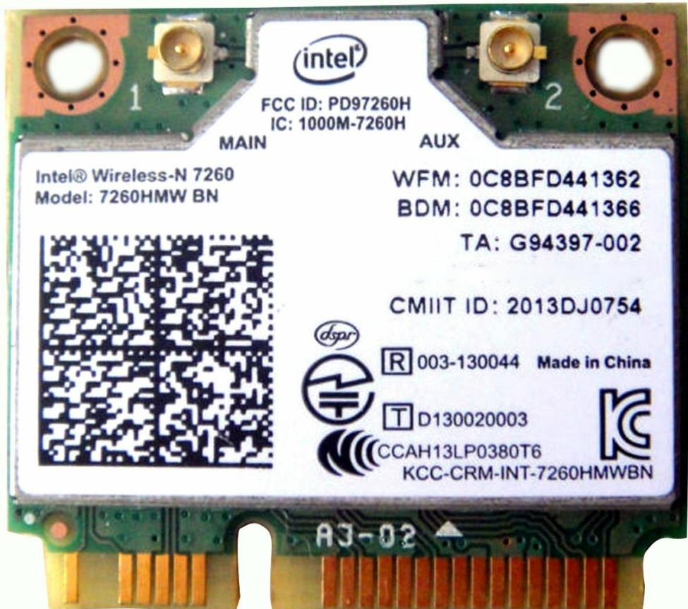
*Image 1: Intel Wireless-N 7260 Half Mini PCI-E Wi-Fi and Bluetooth Card. This image displays the compact form factor of the wireless card, highlighting its connectors and labeling.*
