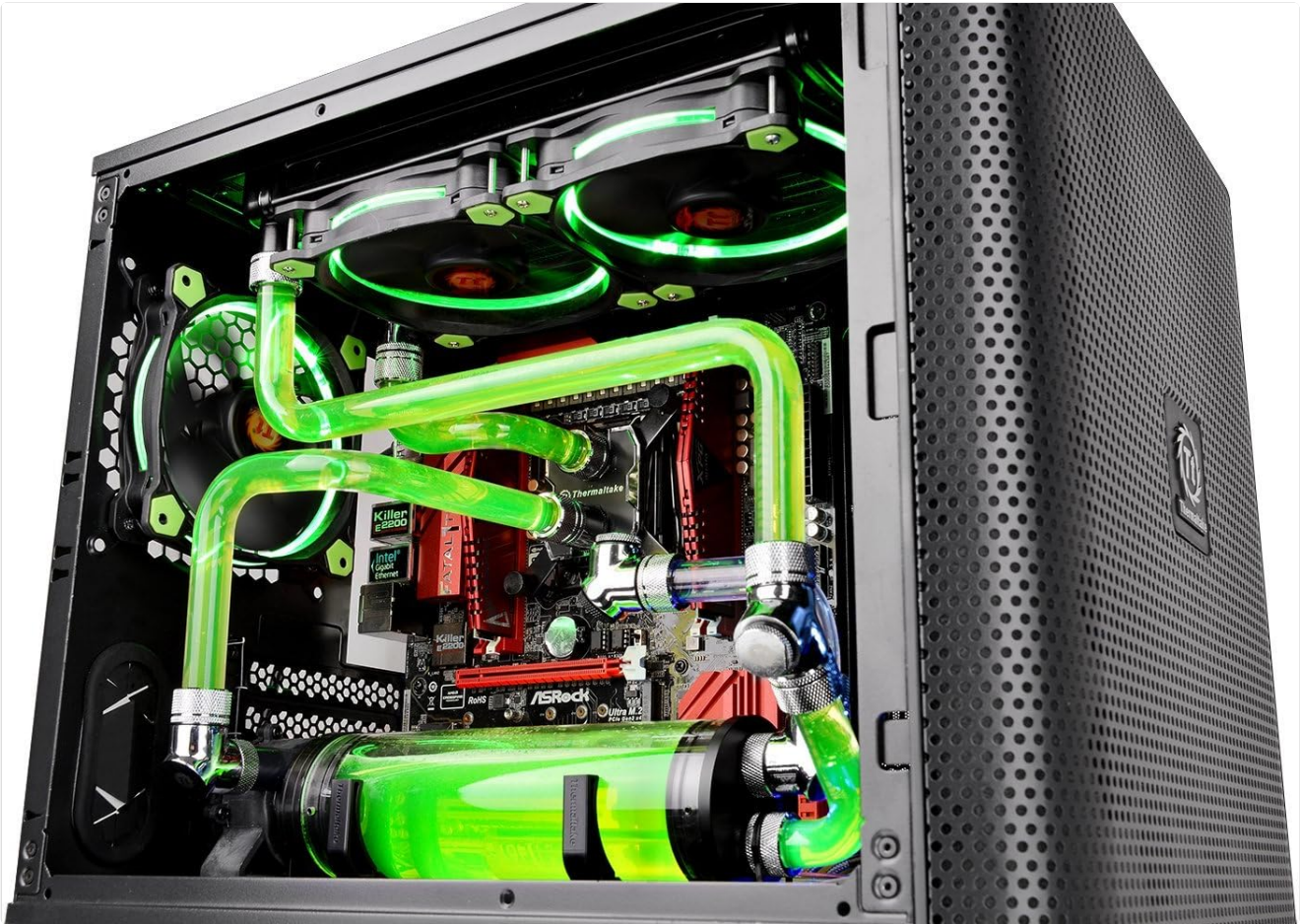
Figure 4.6: Example of a liquid cooling system installed within the Core V21 chassis, demonstrating radiator and tubing placement.
