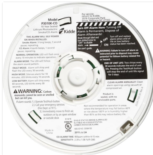
Image 4: The back of the Kidde P3010K-CO alarm, showing the "Turn Off Alarm Here" mechanism and end-of-life instructions.
