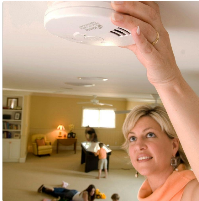
Image 3: A person pressing the central test/reset button on the Kidde P3010K-CO alarm, demonstrating the weekly testing procedure.
