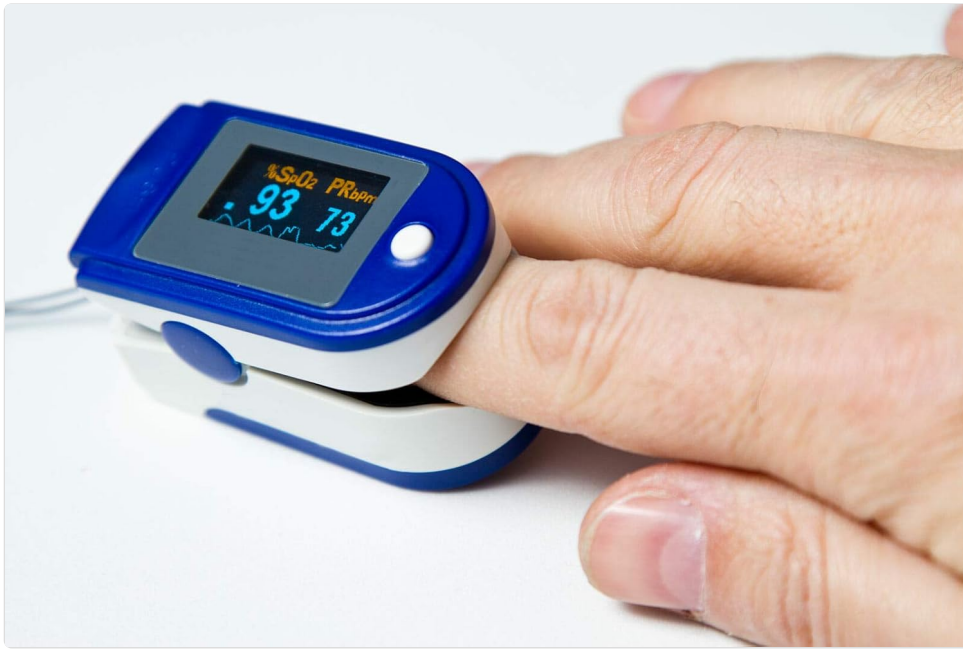
Figure 2: The pulse oximeter correctly placed on a finger, displaying SpO2 and pulse rate readings.
