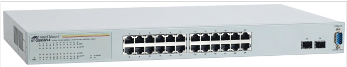
Figure 1: Front panel of the AT-GS950/24-10 WebSmart Switch, illustrating the Ethernet ports, SFP slots, and status indicators.
