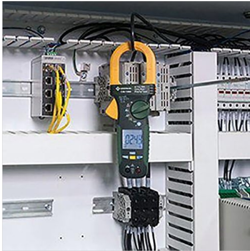
Figure 4.2: The CM-660 clamp meter in use, measuring current by clamping around a single conductor.
