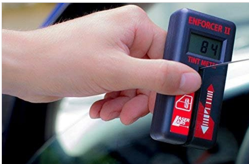
Image: A hand demonstrating the use of the Enforcer II Tint Meter by sliding it onto a car window to take a measurement.
