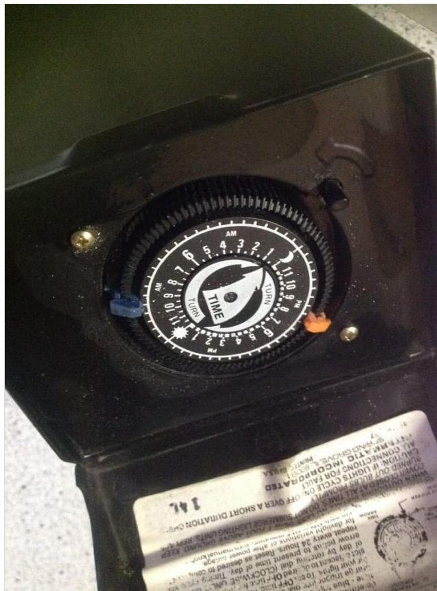
Figure 4.1: Internal view of the timer dial, showing the mechanism for setting ON/OFF times.
