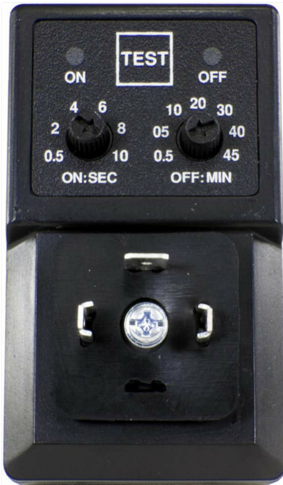
Figure 1: Front view of the YS-720 Electronic Timer, displaying the ON and OFF time adjustment dials and the 'TEST' button. The 'ON' dial controls the duration the valve is open (in seconds), and the 'OFF' dial controls the duration the valve is closed (in minutes).
