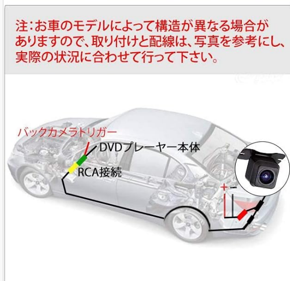
Image 3.1: Illustration of the package contents and a basic wiring diagram for the EONON A0119J Backup Camera.
