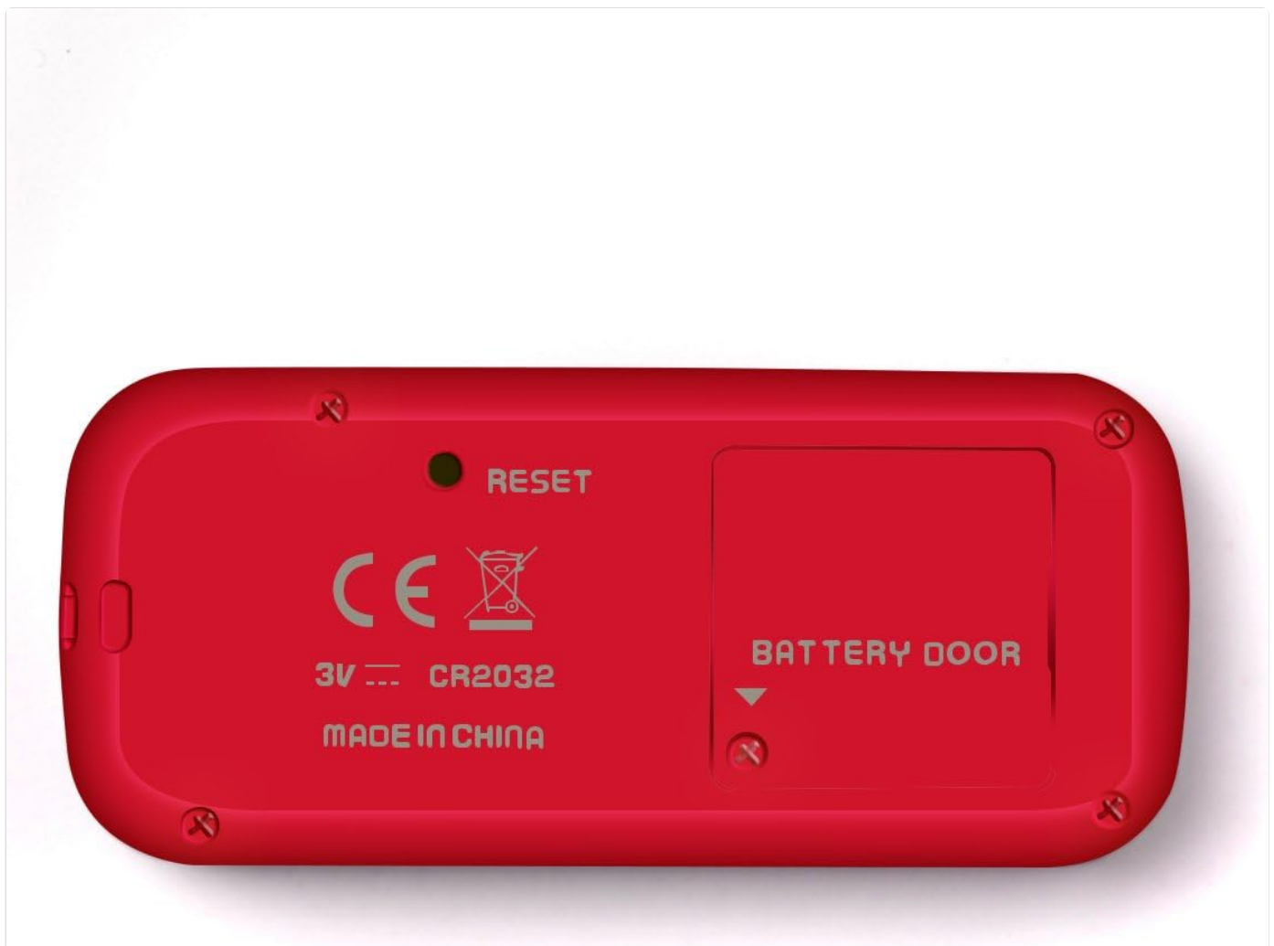
Image 3.1.1: Back view of the activity tracker, highlighting the battery door and reset button.
