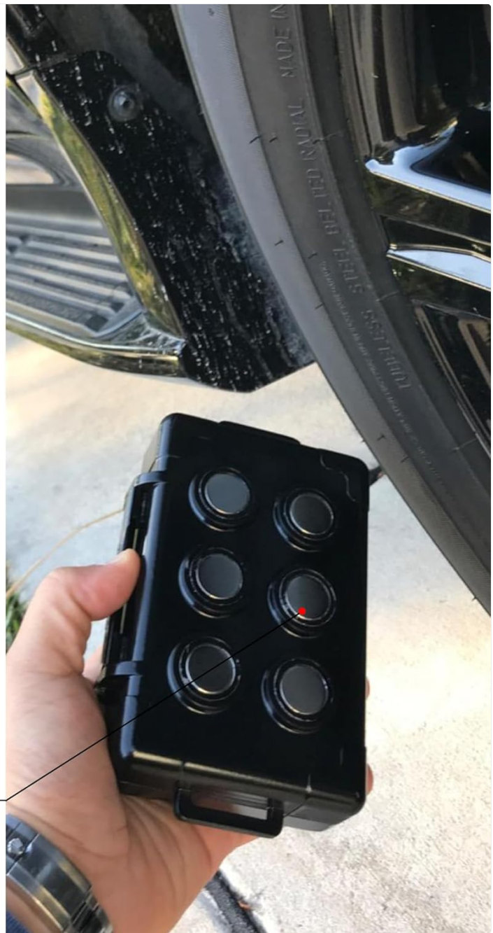
Figure 3: Secure magnetic mounting of the tracker case.
