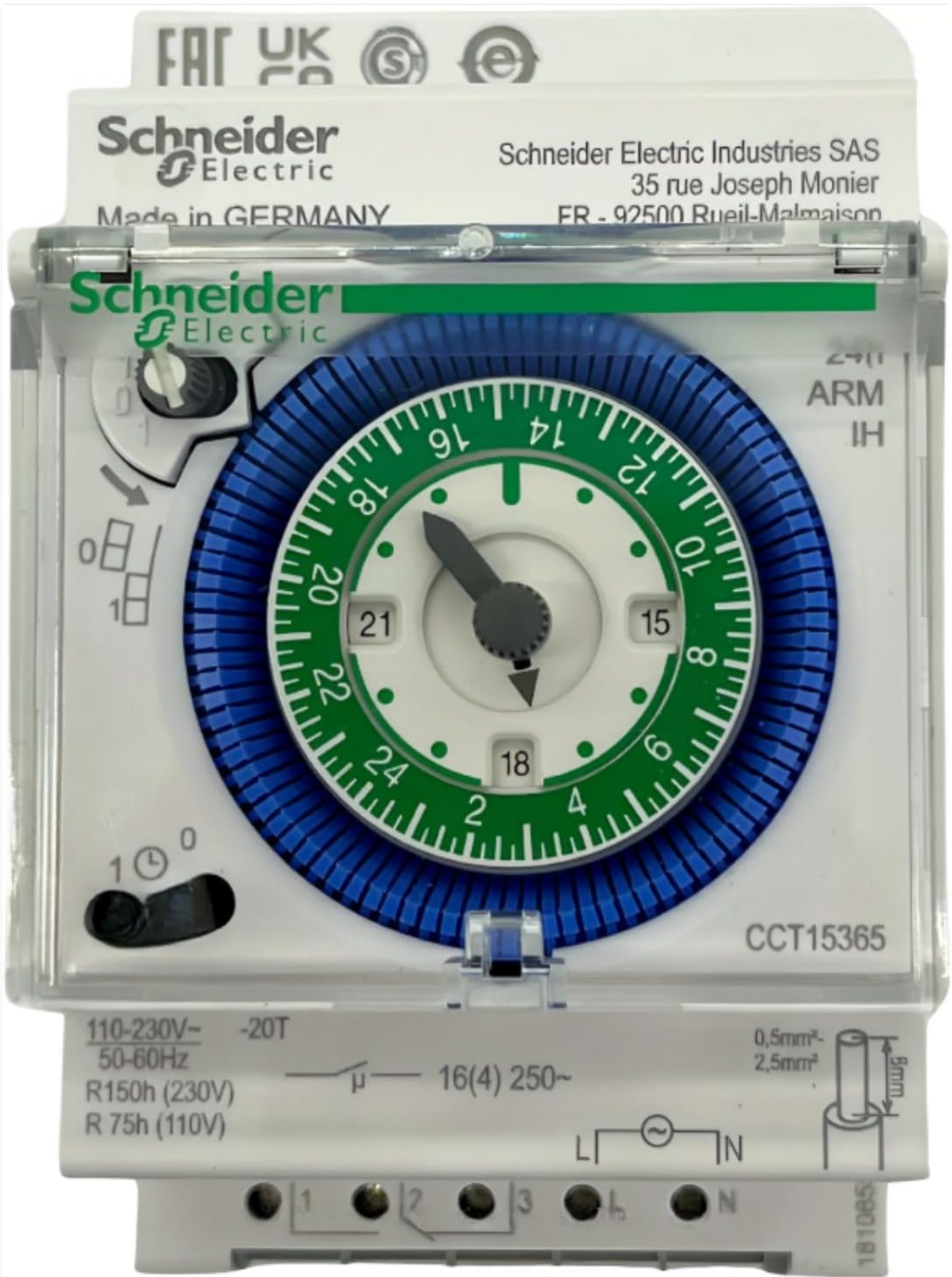
Figure 2.2: Detailed front view highlighting the 24-hour dial and time setting indicators.
