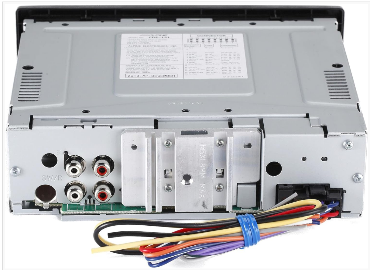
Figure 1: Rear Panel and Wiring Connections. This image displays the rear of the Alpine CDE-151 receiver, showing the main wiring harness connector, antenna input, and RCA preamp outputs. The color-coded wires of the harness are visible, indicating connections for power, ground, speakers, and accessory functions. Ensure all connections are secure and insulated.
