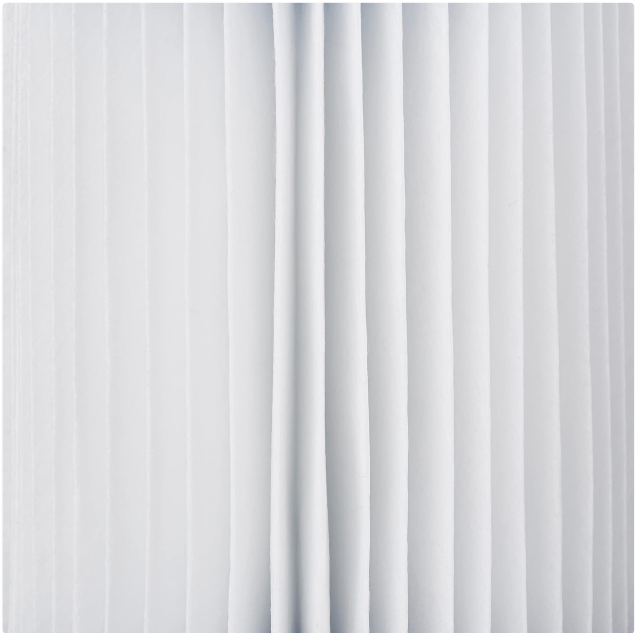
Image: A detailed view of the pleated Dacron material that forms the filtration surface of the cartridge.
