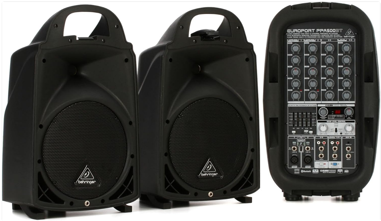
Image: The Behringer EUROPORT PPA500BT system showing the two speaker units and the central mixer unit, which can be detached and stored within one of the speakers for transport.
