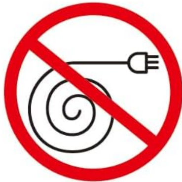
Image 2.2: Warning to fully extend the cord before use to prevent overheating.
