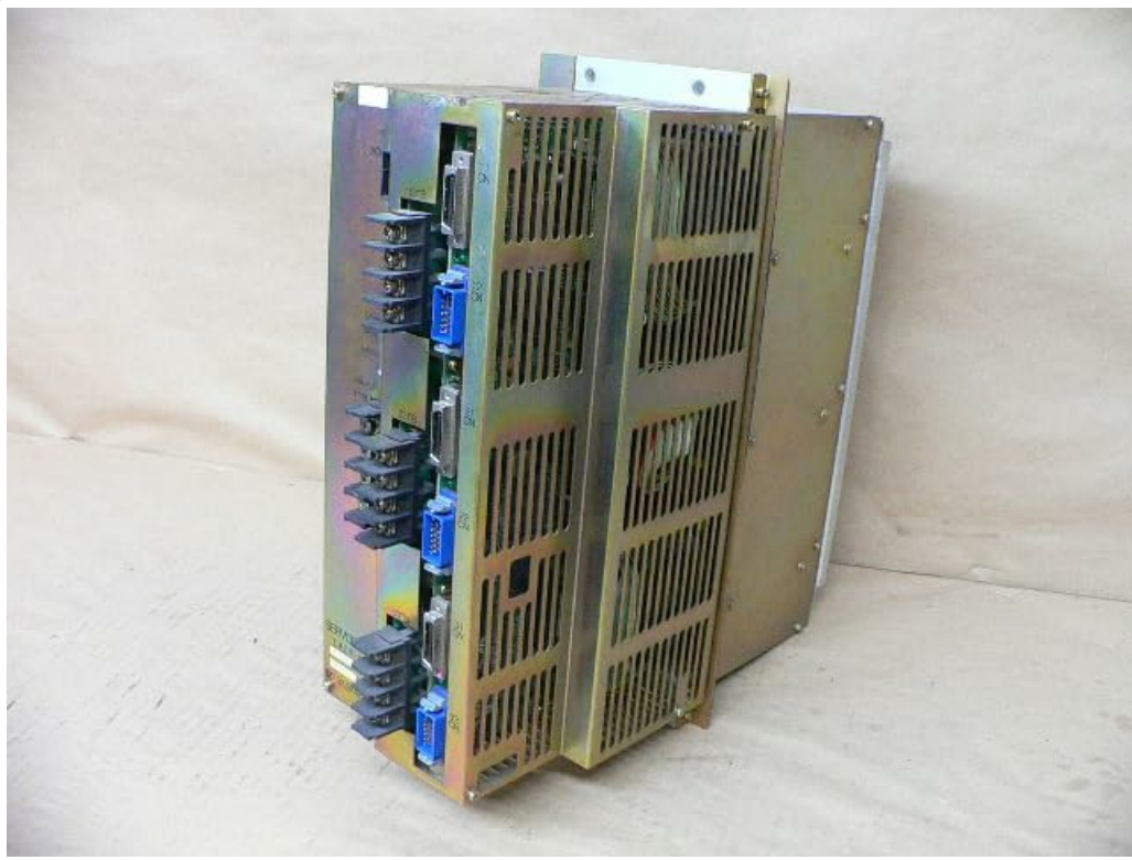
Figure 3.1: General view of the Yaskawa SERVOPACK CACR-IR 151515FB. This image displays the unit from an angled side, showing multiple connection terminals on the left side and ventilation grilles along the top and front surfaces, indicating its industrial design and cooling features.
