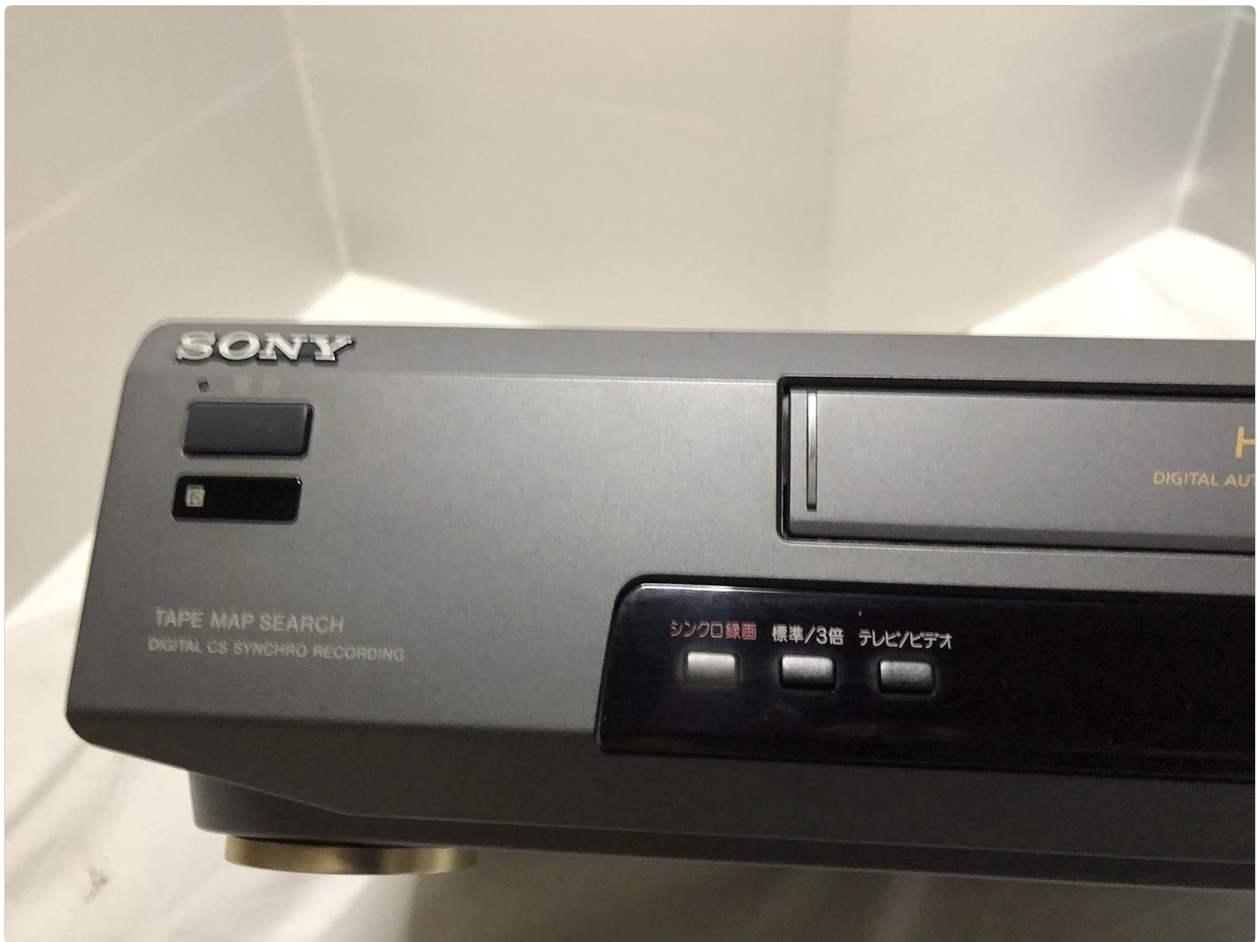
Figure 3: Front left section of the Sony SLV-FT5 VCR. This view highlights the tape loading slot and the 'TAPE MAP SEARCH' feature, which assists in navigating recorded content on a tape.
