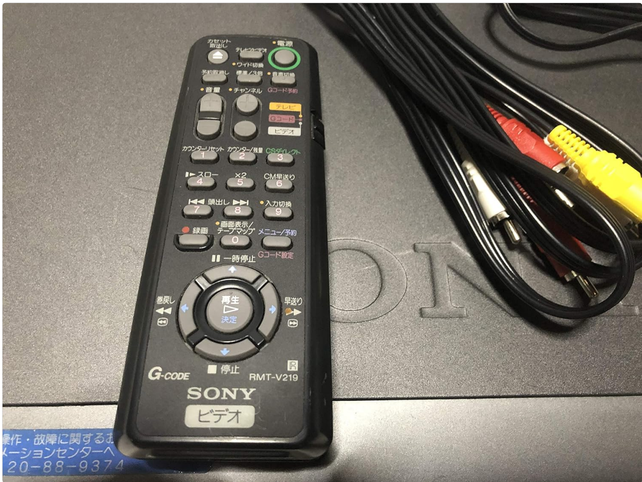
Figure 2: The Sony RMT-V219 remote control, designed for the SLV-FT5 VCR. This image also shows the included RCA audio/video cables, which are typically used for connecting the VCR to a television.
