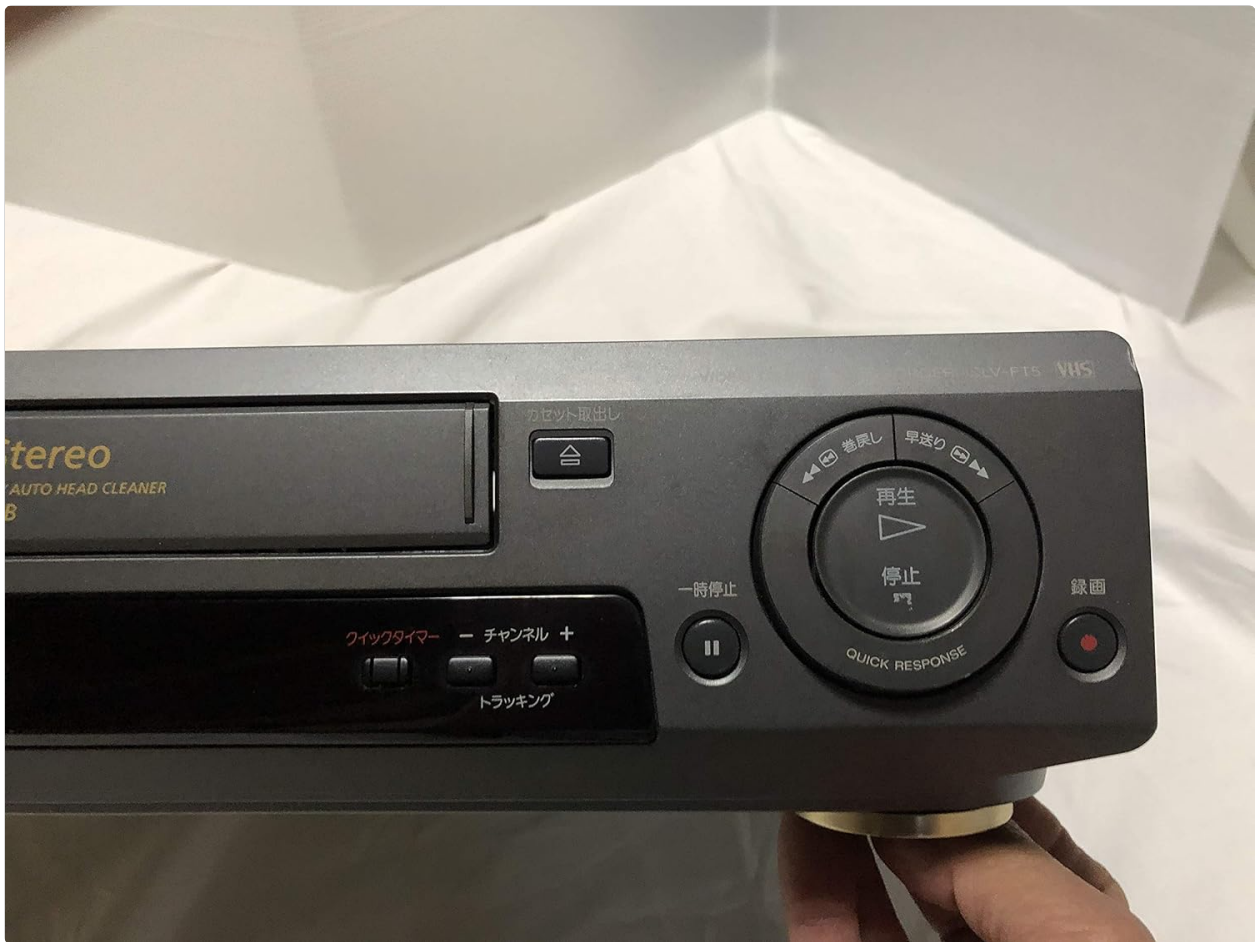
Figure 4: Front right section of the Sony SLV-FT5 VCR. This image displays the main playback controls (Play, Stop, Rewind, Fast Forward, Pause) and additional buttons for 'Quick Timer' and 'Tracking' adjustments.
