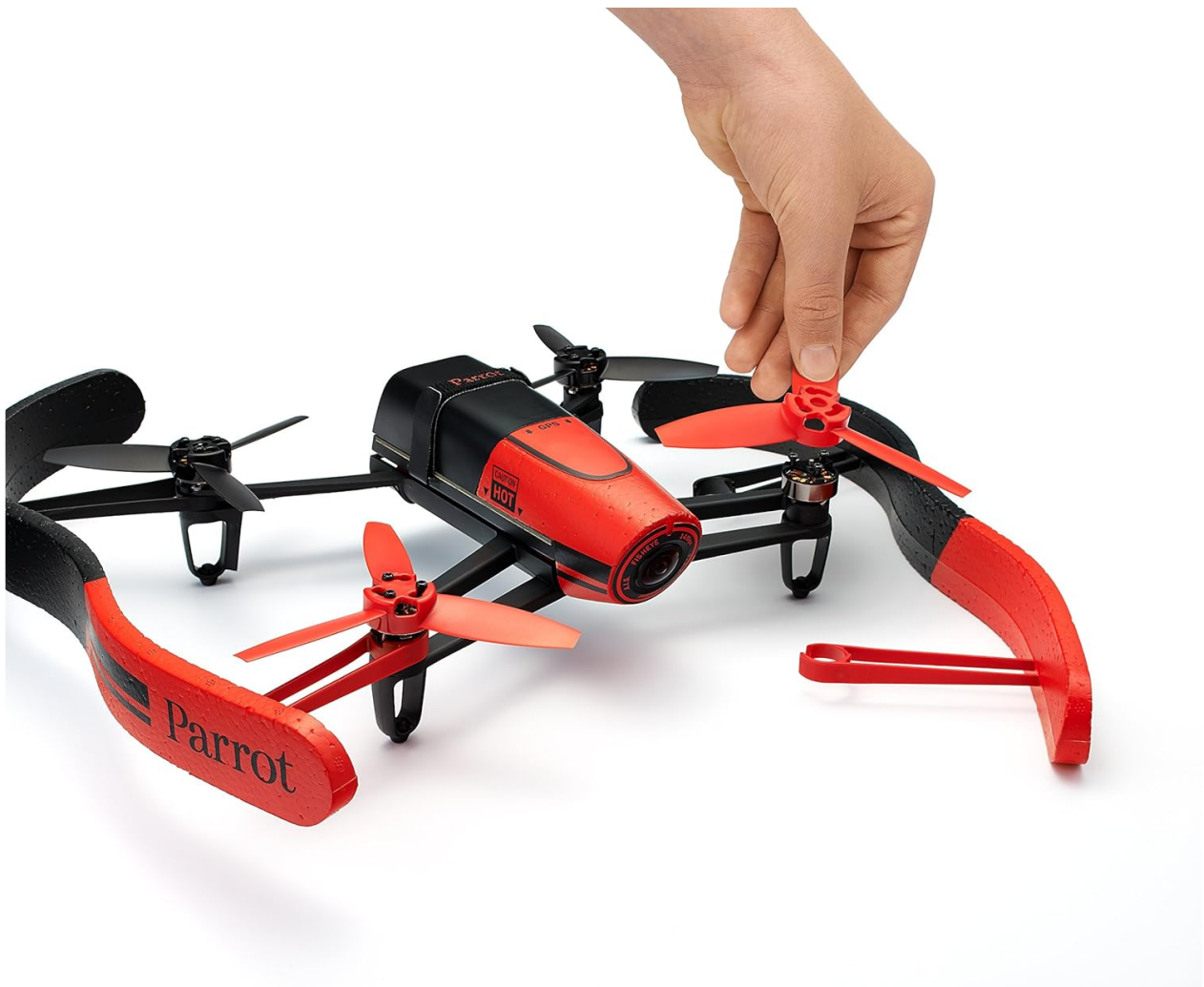
Image 2.1: Proper attachment of propellers to the drone.
