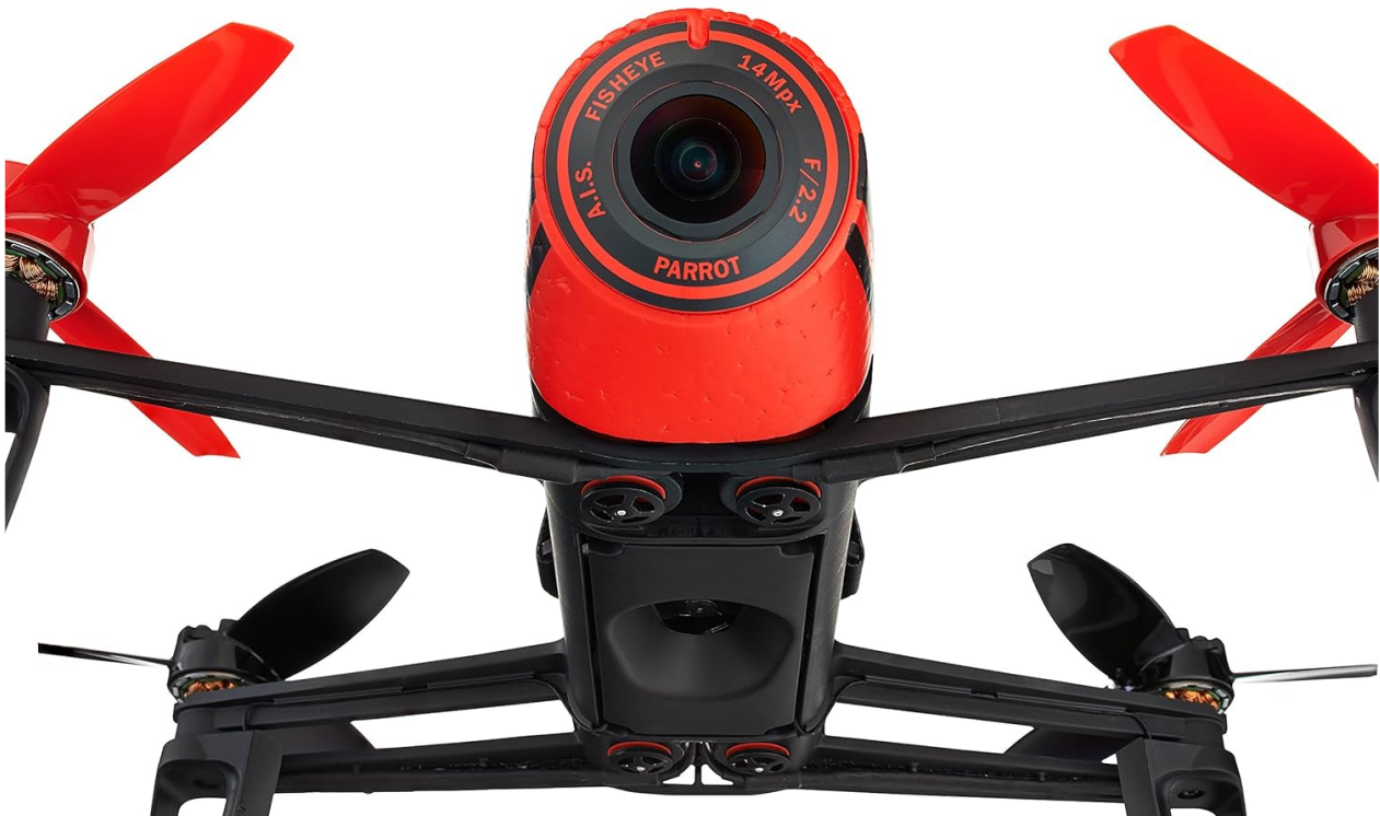
Image 3.1: Detailed view of the drone's fisheye camera.
