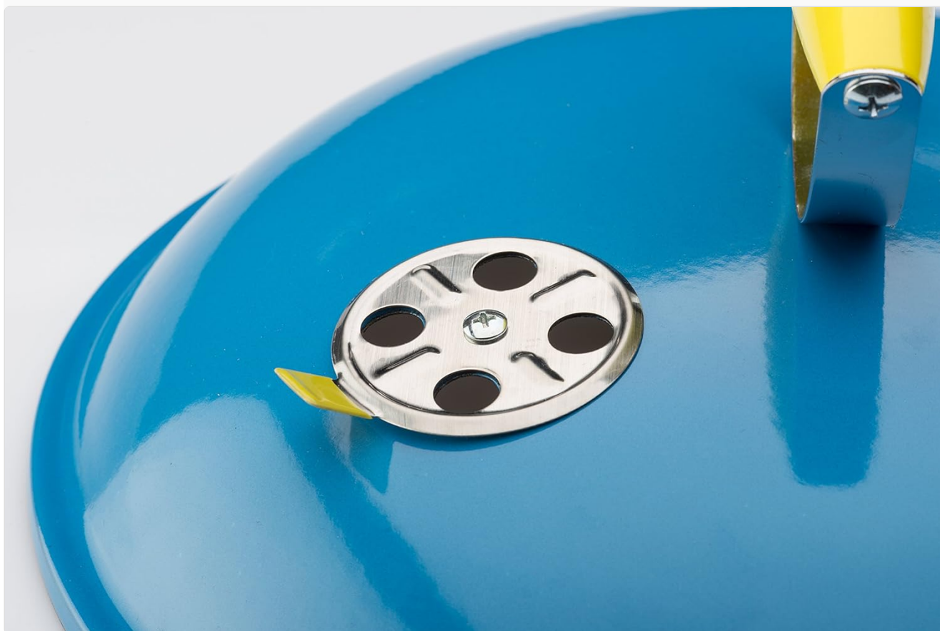
Figure 3: The adjustable ventilation panel on the lid, used to control airflow and regulate the internal temperature of the grill.
