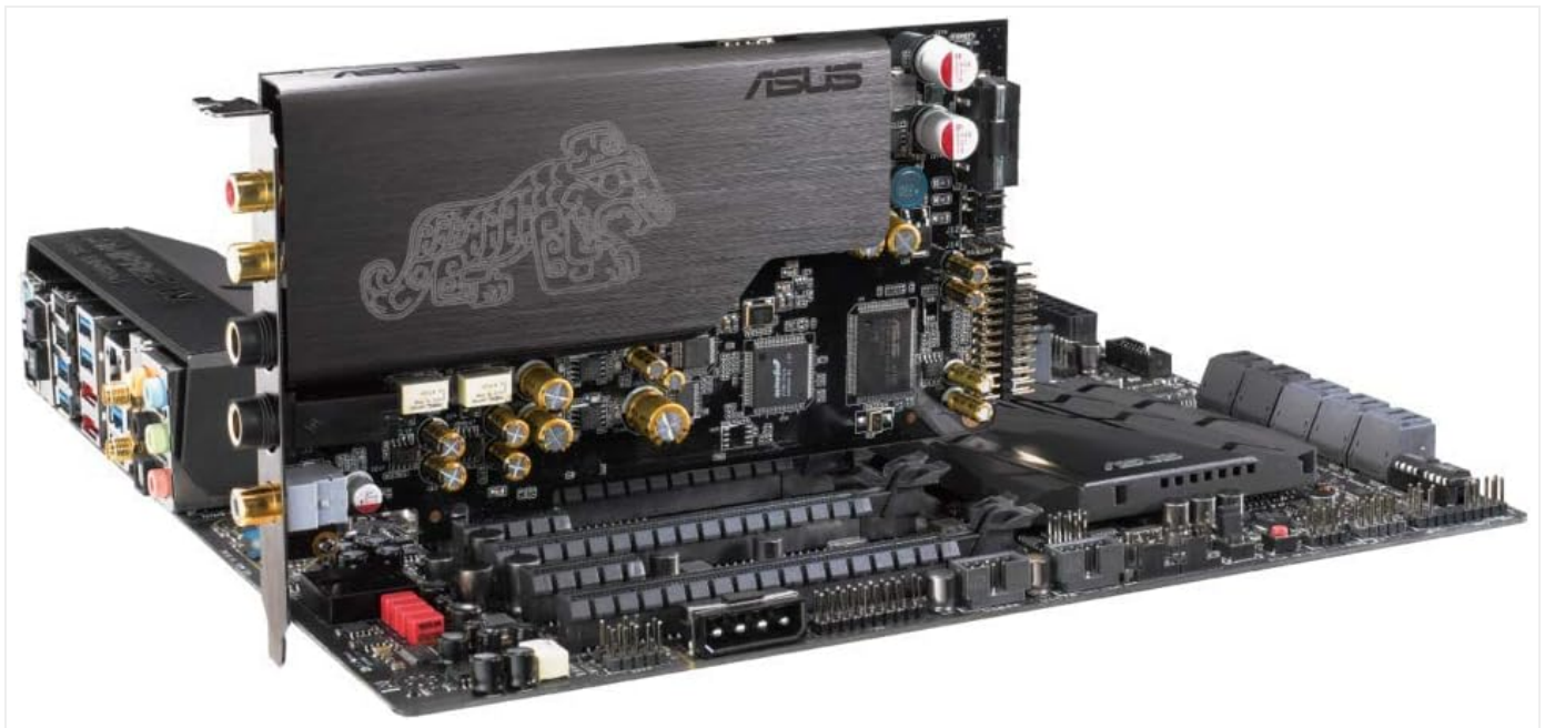
The ASUS Essence STX II sound card installed in a motherboard, demonstrating its physical integration within a PC system.
