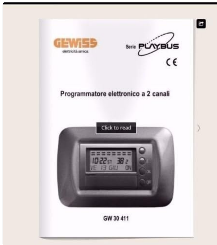
Figure 1: Front view of the Gewiss GW30411 Programmer. The display shows the current time (10:22), day (VE 13 GIU, likely Friday 13th June), and the 'ON' status, indicating an active program. Buttons for navigation and setting are visible on the right side.
