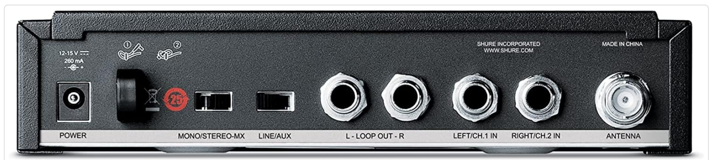
Figure 3: Rear panel of the Shure PSM300 P3T Transmitter, illustrating power input, audio inputs (L/R), loop outputs, and antenna port.
