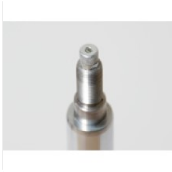
Image: Detail of the damping force adjustment mechanism.
