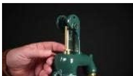
Figure 3: Detail of the brass valve and self-draining mechanism at the base of the stand-pipe.
