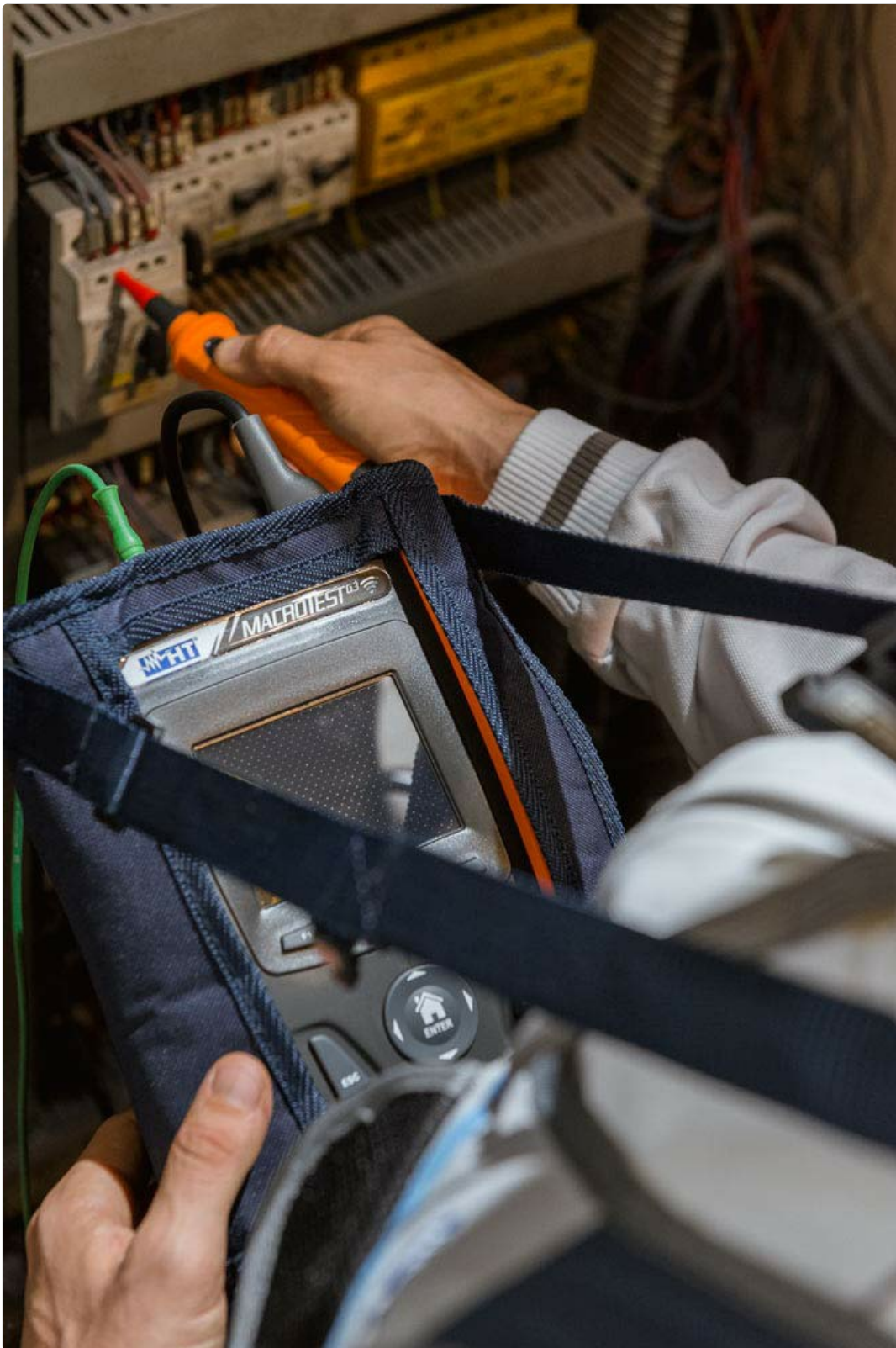
Figure 3: A user operating the MACROTESTG3 while performing tests on an electrical panel. The tester is shown in its protective carrying case, demonstrating its use in a professional setting.
