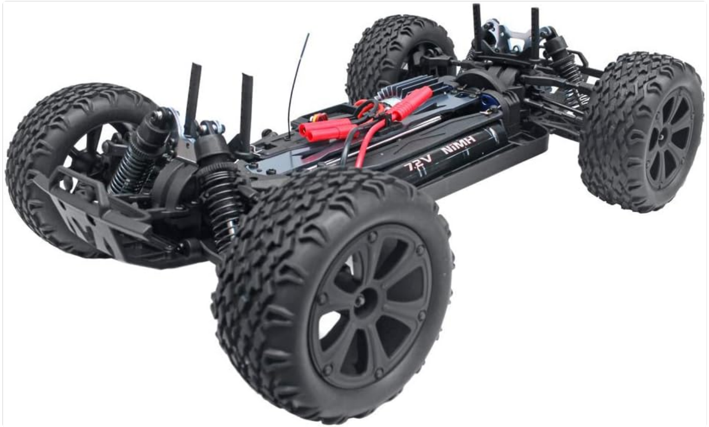
An overhead view of the Blackout XTE chassis without the body, showing the battery compartment and electronic components.
