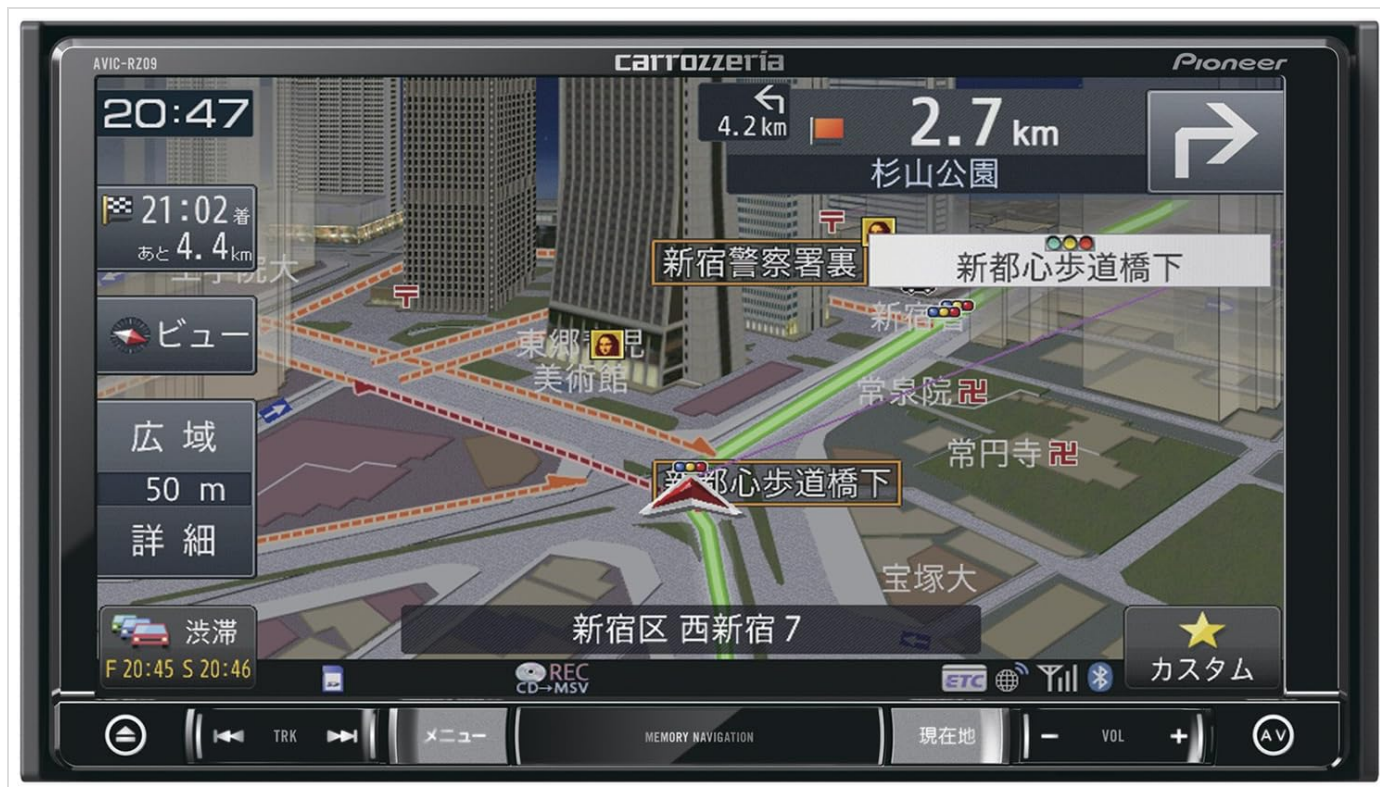
Image 3: Close-up of the AVIC-RZ09 screen. This close-up image focuses on the 7-inch wide VGA display, showcasing its map interface. The screen clearly shows a navigation route, current traffic conditions, and points of interest, demonstrating the system's detailed visual guidance capabilities.
