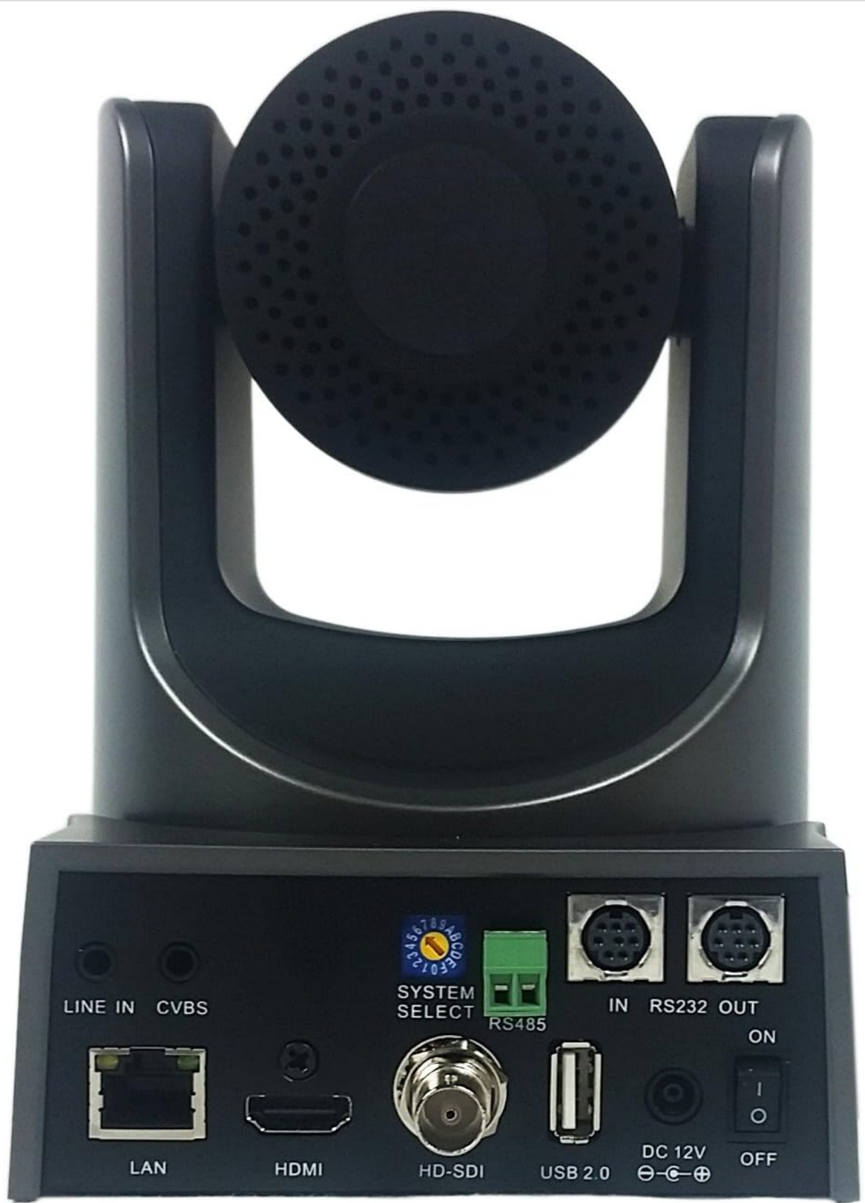
Figure 3: Rear panel connections of the PTZOptics 12X-SDI camera. This image details the array of ports available for connectivity, including LAN, HDMI, HD-SDI, USB 2.0, DC 12V power input, RS-232 In/Out, RS-485, CVBS, and Line In audio.
